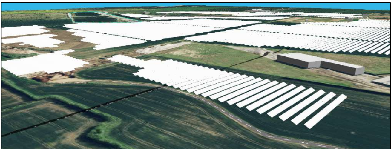
Figure 2.2: Fixed Solar Panels – CadnaA Model
